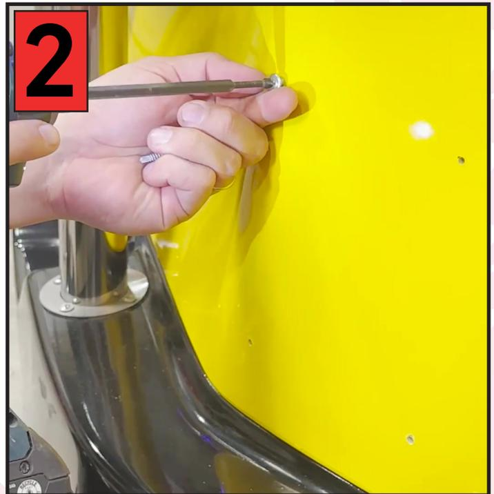
**2** Position the wipes dispenser aligned with the holes and secure it by tightening the four screws.
